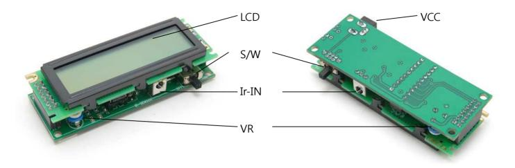
\* LCD : Displaying Infrared Ray (Ir) Data.
