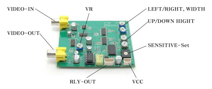
\* VIDEO-IN : video input terminal.\* VCC : power input DC 5V.\* RLY-OUT : relay contact output.
